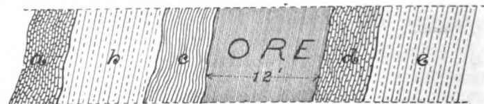
Fig. 27.—Section showing ore body, north end of Crowder's Mountain.
